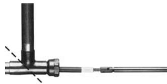
**Replace 90 Degree Elbow**—Cut out the elbow fitting without damaging the ends of the pipe. Insert the Jet Swet™ tool into the pipe and tighten until the water stops. Remove both halves of old 90 degree elbow. Slide a T-fitting with a FIP adapter over the Jet Swet™ and solder them onto the pipe. Remove the Jet Swet™ and plug FIP adapter.
