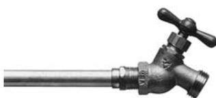
**Replace Restricted Port or Regulatory Valves**—Shut off water supply. Completely cut off old valve. Insert Jet Swet™ to shut off draining water. Solder on a male adapter. Replace with any threaded valve.
