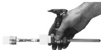
**Repair PVC Pipe**—the Jet Swet™ is the ideal tool for repairing PVC pipe. This technique allows the plumber to glue PVC pipe in a water-free environment. Works on Sch. 120 and Sch. 40 pipes.
