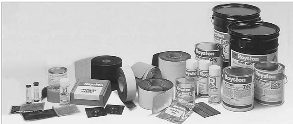
**Royston PatchRight®:** Is a sealing system designed for quick, permanent repair of leaking, low-pressure steel gas lines with maximum pressure of 3 psi. Each kit contains butyl rubber patch, a flexible neoprene tape, and a resin impregnated fabric. PatchRight maintains outstanding electrical resistance and physical properties without deterioration over time or exposure to corrosive underground environments.
