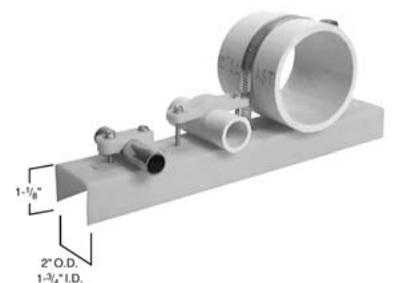
**STANDARD** A-507 and A-607 Channel is 1-1/8" x 2" x 7" and comes with holes and slots for use with the P-552 stainless steel band and/or the 1/2"–3/4" or 1"–1-1/2" clamps.
